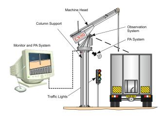
The system can also be customised to suit a site's requirements, which may include the addition of an observation system, traffic lights, column support, PA system, purging system, tanker mode, or dual lane control.
