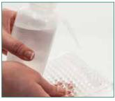
7. Repeat steps 3-5 by dumping out the liquid. thoroughly washing the wells and tapping dry.
