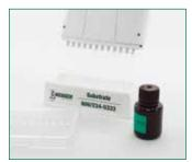
8. Transfer 100 µL substrate from reagent boat to antibody wells using 12-channel pipettor. Incubate for 10 minutes. Mix for 20 seconds by sliding back and forth on a flat surface.
