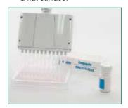
6. Transfer 100 µL conjugate from reagent boat to antibody wells using 12-channel pipettor. Incubate for 10 minutes. Mix for 20 seconds by sliding back and forth on a flat surface.
