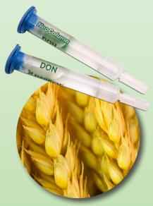
A robust, highly effective immunoaffinity column for use in the detection of DON in a broad range of foodstuffs and in animal feed. Data obtained from an extensive testing program demonstrates high performance of NeoColumn DON which can be used for a purification step prior to HPLC, GC-MS, ELISA and other analytical methods. Available in wide bore format.
