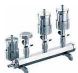
Three-place filtration unit with vacuum filter holders made of stainless steel, 50 mm diameter, self sealing. The filter holder are connected via a gliding socket to the filter holder and therefore easy to remove. A combination of filter holder of 50 mm and 80 mm diameter is possible. Due to its small dimension the filter holder is especially suitable for working in safety workbenches.
