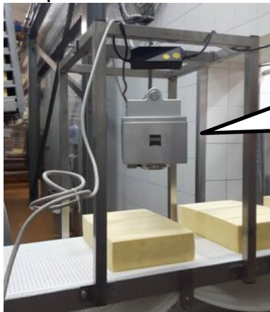
Figure 1: Corona process over conveyor
