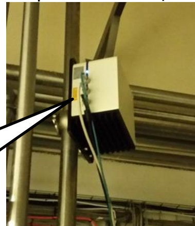
Figure 2: Corona extreme on GEA flange
